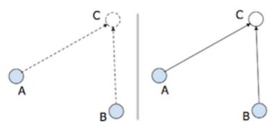
**Figure 18.** Basic learning process: If connections AC and BC are active at the same time, and if their joint activation is strong enough to activate C, they both get strengthened and the threshold of C is adjusted
