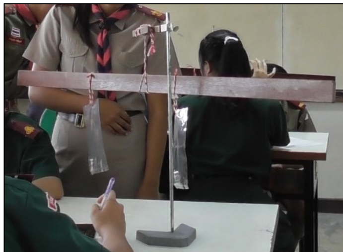
Figure 1. A lever made from a meter ruler hung on a test-tube stand.
