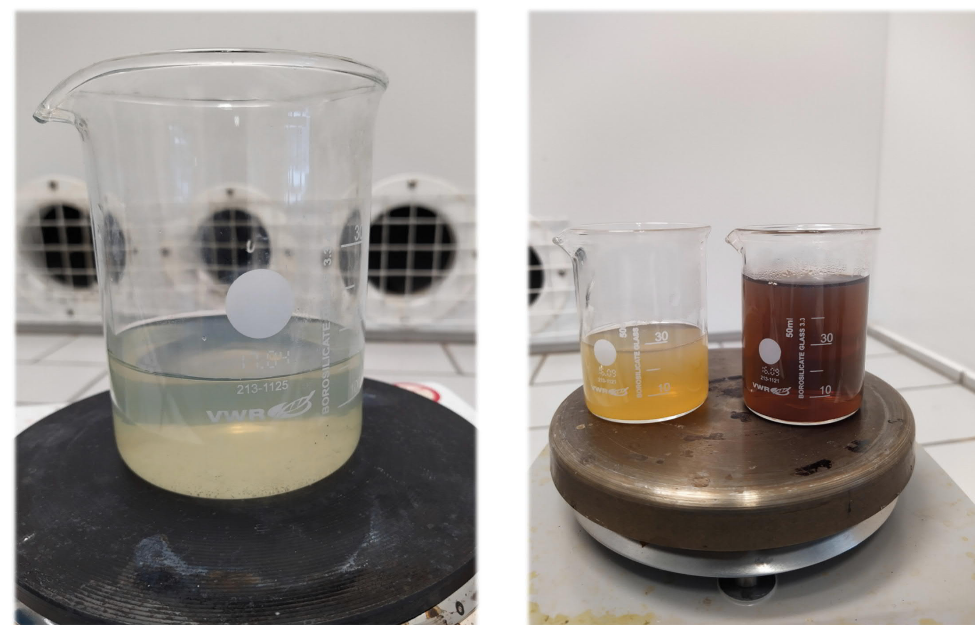
Figure 1 & 2. On the left, the extracted and filtered watermelon rind extract is presented. On the right, two different samples of silver nanoparticles are presented exhibiting the spectroscopic phenomenon: localised surface plasmon resonance (LSPR).
